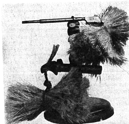
Appleby's "knotter," which became the self-binder.
